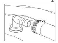
2. Slide a hose clamp on to the bypass hose (from the relief valve), then with a twisting motion, slip the bypass hose over the fitting on the top of the tank. Slide the hose clamp to the end of the hose and secure.
