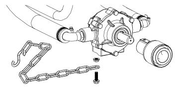
5. The roller pump IS included with the assembly. Attach the adapter, torque chain and S-hook to the pump as needed. It is intended for pump to be mounted directly to the tractor PTO. Torque chain needs to be secured to the tractor to keep your pump from spinning.
