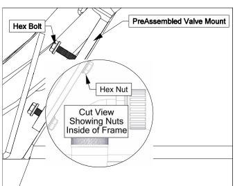
Install the preassembled tee valve sub-assembly to the
