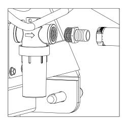
3. Using a good quality thread sealant, carefully thread the 1" fitting into the strainer. Find the 1" x 36" pump feeder hose. Slip a hose clamp onto the ends of the hose. With a twisting motion, slip the hose all the way onto the fitting and secure with the hose clamp.
