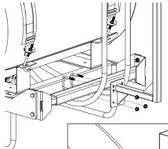
8. Attach the boom buster bracket to the telescoping brackets, using the two square u-bolts and 4 whiz nuts. The telescoping brackets are already mounted to the 3-point frame.
