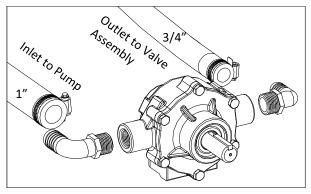
4. Using a good quality thread sealant, thread 1" fitting into the inlet (IN) side of the pump and the 3/4" fitting to the outlet (OUT) side of the pump. With a twisting motion, attach the other end of the 1" hose to the 1" fitting on the inlet to the pump. Slip a 3/4" hose clamp onto the 3/4" hose coming off the valve assembly and with a twisting motion, attach the 3/4" hose to the output side of the pump and securing with the hose clamp.
