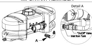
This sprayer comes with an On/Off (shut-off) valve located at the inlet location of the tank, towards the underside. (See Detail A). Make sure the valve is in the "open" position before using sprayer.
