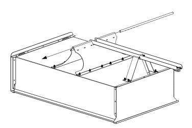
Step 4: Slide the axle through the axle housing and the
