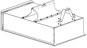
Step 3: Affix yoke brace to the cart body, using (4) round Head machine screws. Secure with lock nuts.
