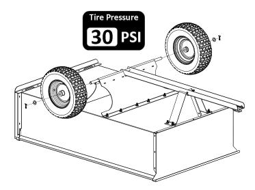
Step 5: Center the axle within the axle housing and place wheel over axle, followed by machine busing on the outside of the wheel.
